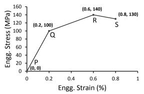
The toughness of the material (in MJ/m<sup>3</sup>) is \_\_\_\_\_
